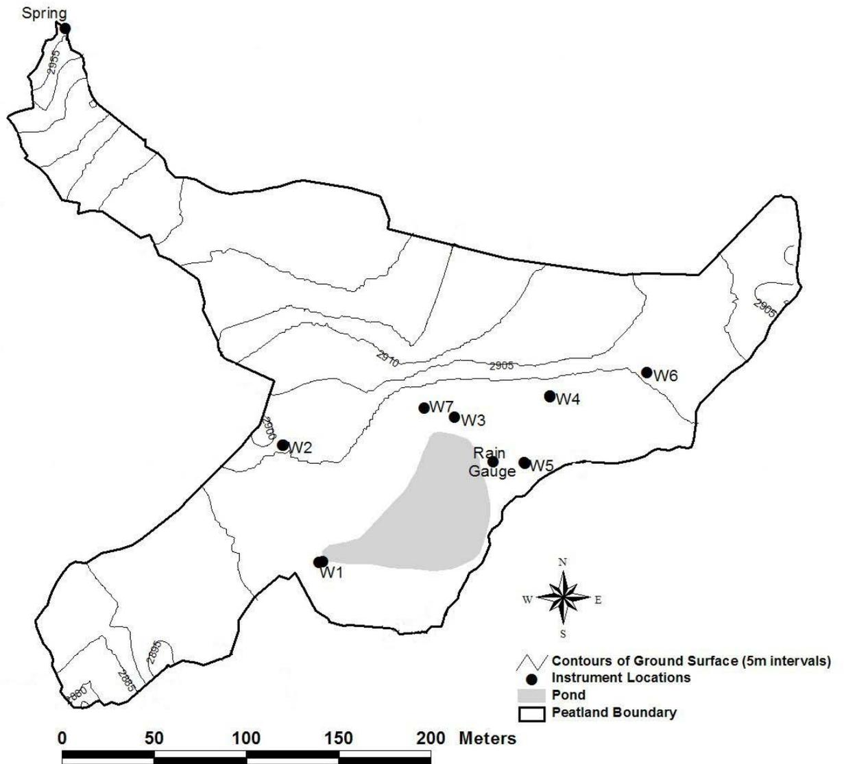
**Figure 1.** Topographic map of Mt. Emmons fen. Well 1, a staff gauge in the fen pond, is located near the pond outlet. Monitoring wells 2-7 are also shown. Contour interval is 5 meters. The fen is 15.1 acres (6.1 hectares) in size.
